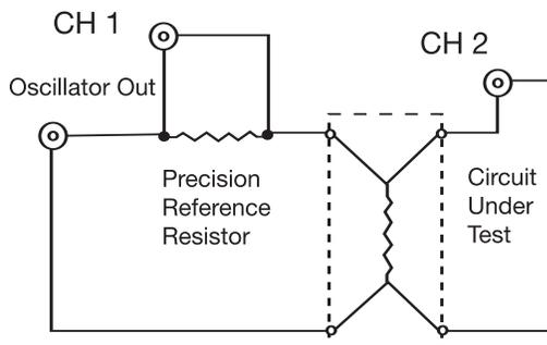
The user selects a component type, or an equivalent circuit, and a starting frequency. For single-component measurements, the starting frequency is the test frequency. For equivalent circuits of two or three components, the starting frequency is automatically varied to locate corner and resonant frequencies used to calculate the component values.
