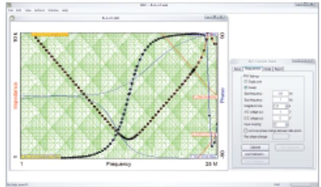
Measured values of components of the circuit under test are displayed on the screen. If the user defines minimum and/or maximum values for any component and measured values are not within specified limits; the system “beeps” and highlights the out-of-spec values.
